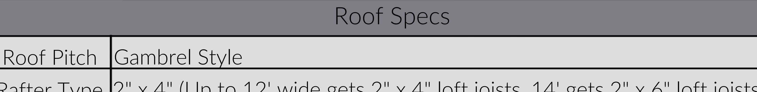
Rafter Type 2" x 4" (Up to 12' wide gets 2" x 4" loft joists, 14' gets 2" x 6" loft joists).
